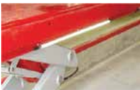
Optional Shatterproof LED 24v Runway lighting
