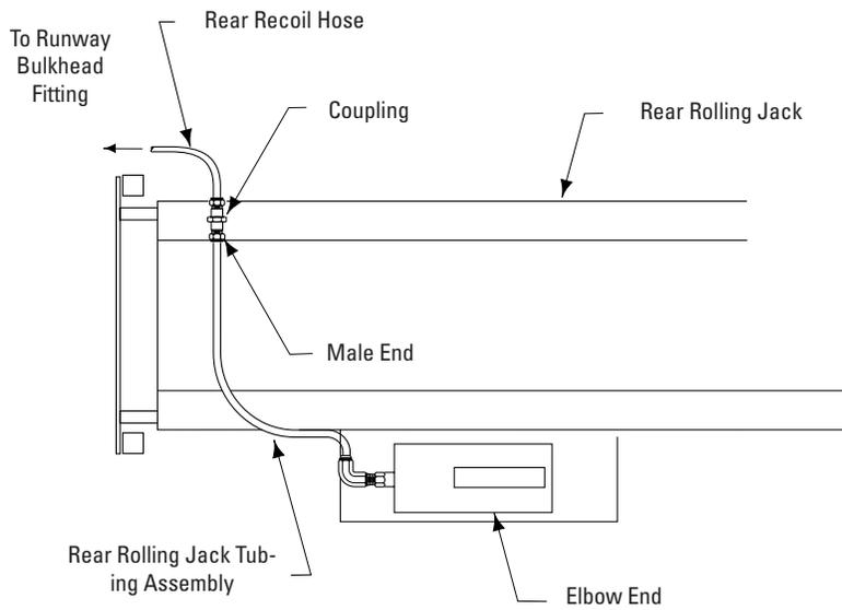
**Fig. 31 REAR ROLLING JACK TO RECOIL AIR HOSE**
