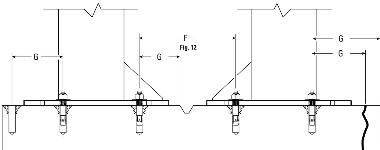
**\*The supplied concrete fasteners meet the criteria of the American National Standard "Automotive Lifts - Safety Requirements for Construction, Testing, and Validation" ANSI/ALI ALCTV-2011, and the lift owner is responsible for all charges related to any additional anchoring requirements as specified by local codes. Contact customer service for further information at: 800.423.1722**
