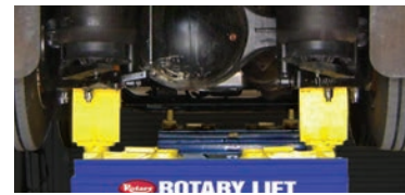
Example of adjustment range and rotated adapters with an off-set transaxle.
