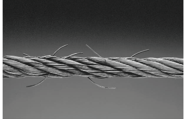
Cable With Broken Wires
